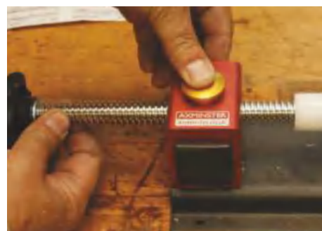
Pressing the gold button overrides the thread for fast adjustment
